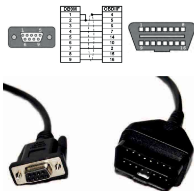
DB9-Male to OBDII-Female Cable
